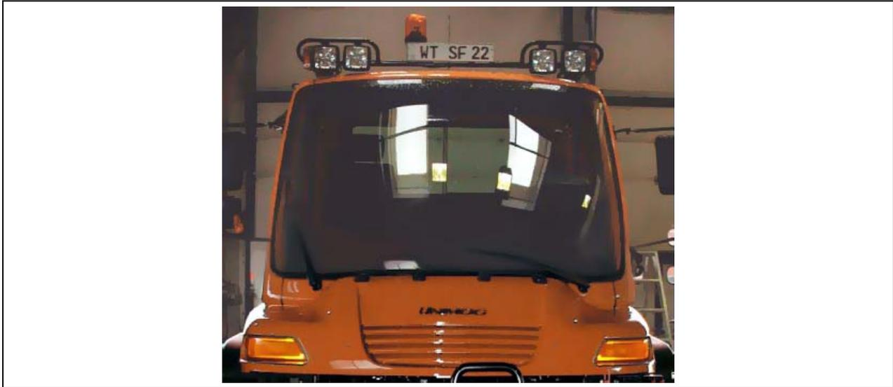
**Example for a roof-mounted light bar. Light bar is not available ex factory!**
